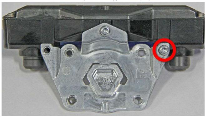
3. Loosely install the LH screw that secures the mounting plate to the camera. Do not torque to screw at this time.
