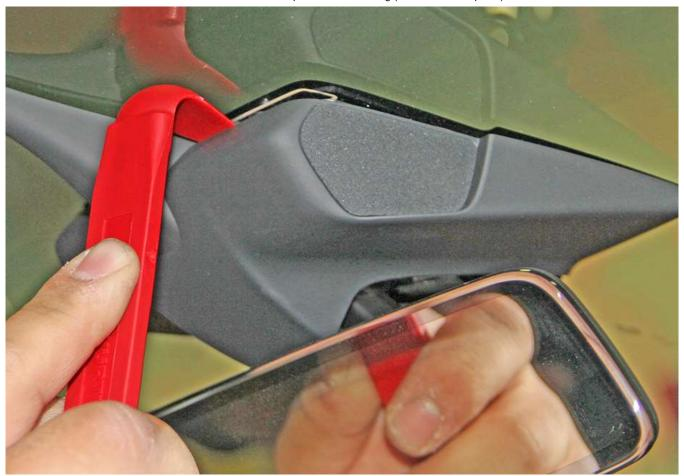
4. Release the screws that secure the mirror bracket carrier to the glare shield (torque 0.8 Nm).
