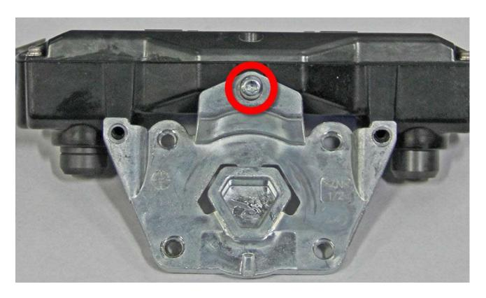
2. Loosely install the RH screw that secures the mounting plate to the camera. Do not torque screw at this time.
